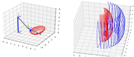
Fig. 2. Left: Simulated LSMS Gantry Constructing a Habitat Shell, Right: Workspace bounds of the LSMS Gantry Printer
