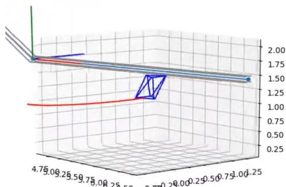
Fig. 3. Underslung Stewart Platform Articulating to Respond to Sway in the LSMS
